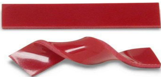
Figure 2. Shape Memory Polymer-SMP, Vybornem: the nanostrip dimensions: 5 x 25 x 125 nm; Presentation of the Shape Memory Polymer after 25 tests, max. Strain 100%;
